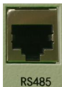
Figure 2-2 Controller device RJ45 interface (RS485 communication protocol)
